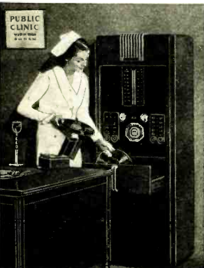
A modern 2-channel hospital sound installation. It provides patients with radio-phono, entertainment. Unit also includes talk-back facilities—the speakers act as "mikes"; see page 688.
