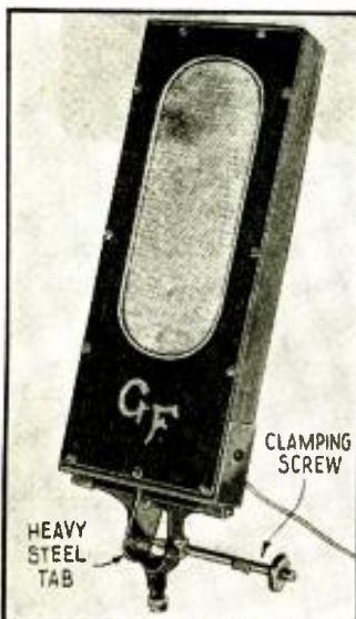
Fig. A, left. The appearance of the complete velocity microphone with its "line" transformer all mounted in a neat case are readily seen.
