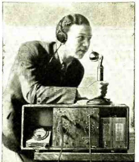
Below. The remote unit; note the new type W. E. dynamic microphone.
